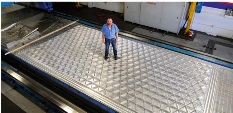
**Fig. 3** Image of lightweight isogrid panel (<http://www.amrofab.com/>)
