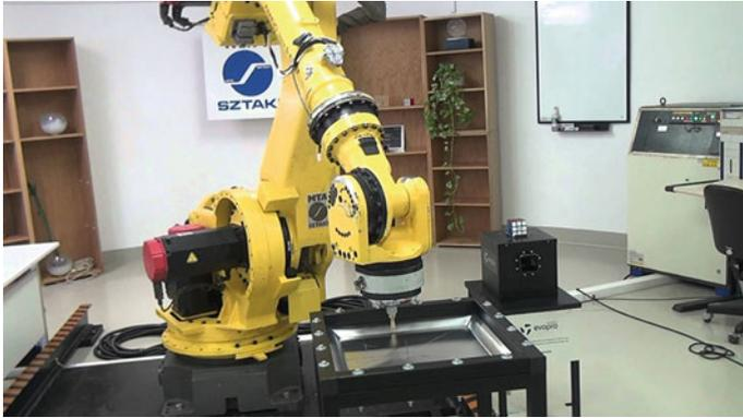
**Fig. 1** Robotically controlled ISF processes ([http://i1.ytimg.com/vi/xcg08U\\_Y4PI/maxresdefault.jpg](http://i1.ytimg.com/vi/xcg08U_Y4PI/maxresdefault.jpg))
