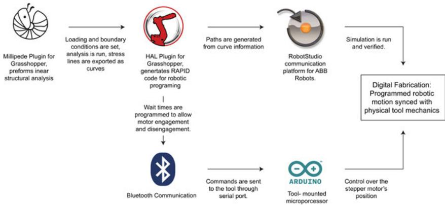
Fig. 10 Workflow for toolpath generation and motor control
