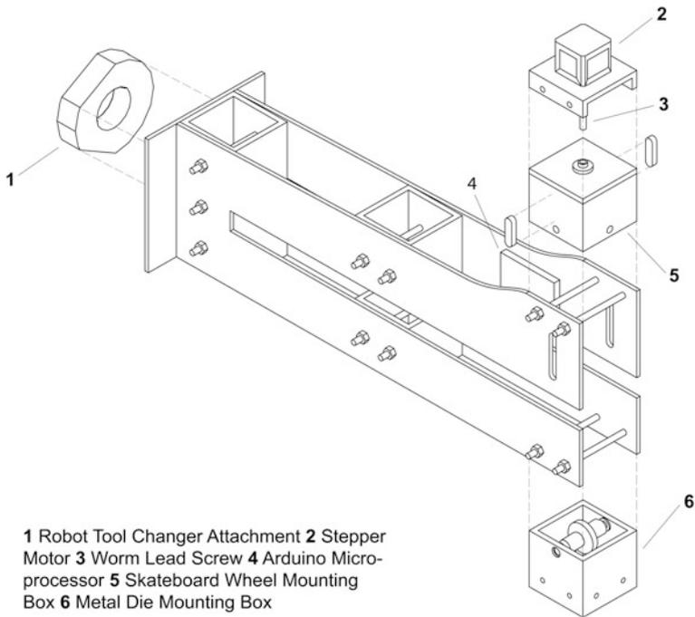
Fig. 4 Diagram of tool affixed to robot
